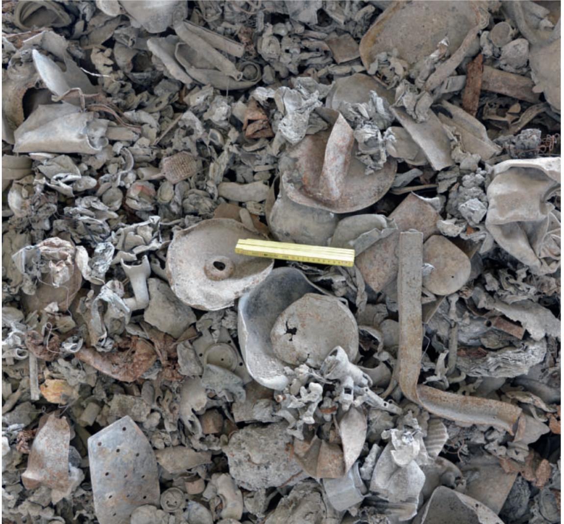
ger than 3 mm contained in the bottom ash are recovered
