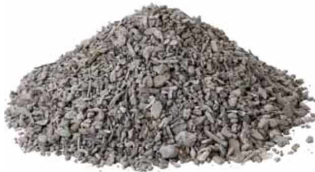
Mix of light and heavy metals from supersort®fine : fine fraction ( <3\text{mm} )
