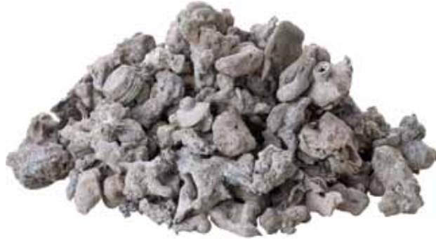
Mix of light and heavy metals from supersort® : coarse fraction ( >3\text{mm} )
